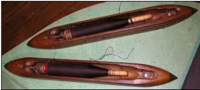
Figure 1: John Kay's flying shuttle
